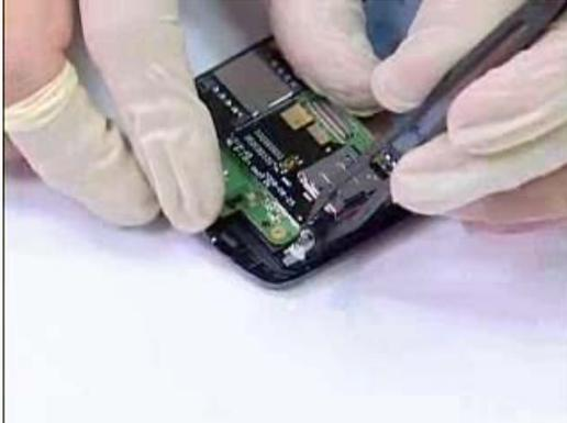
Assemble the vibrator on bezel as shown
