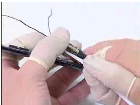
Connect the LCM connector with main board as shown.
