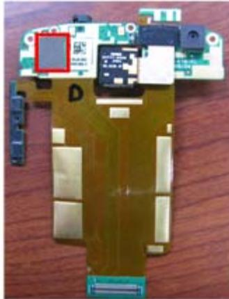
Paste a gasket on rigid flex board as shown.
