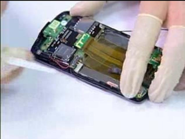
Put the cable into the slot of bezel
