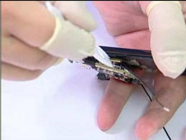
Disconnect the BT/WLAN coaxial cable from MAIN BOARD as shown.
