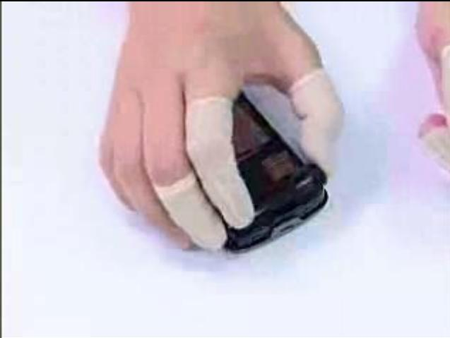
Assemble the antenna cover on housing
