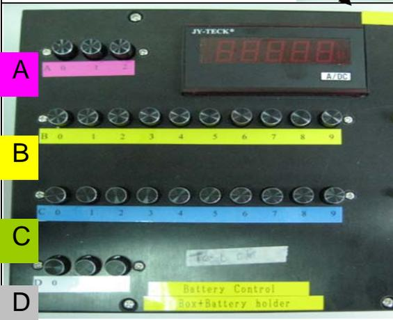
2. Set up each button by row A~D according to product specification Following is an setting for Diamond
