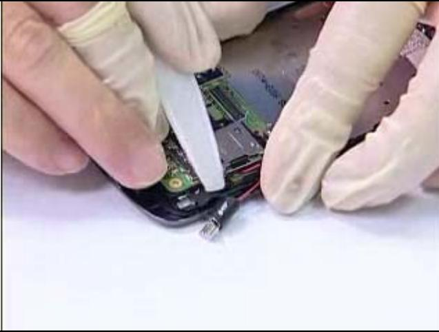
Remove the Vibrator as shown.
