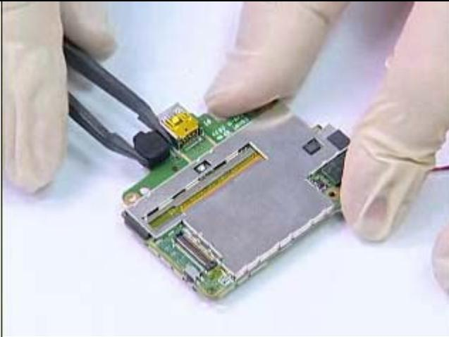
Remove the Microphone Rubber from MAIN BOARD.
