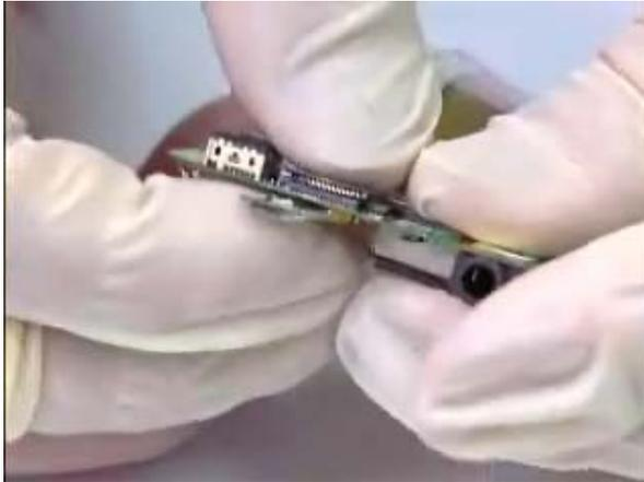
Assemble the Main camera as shown
