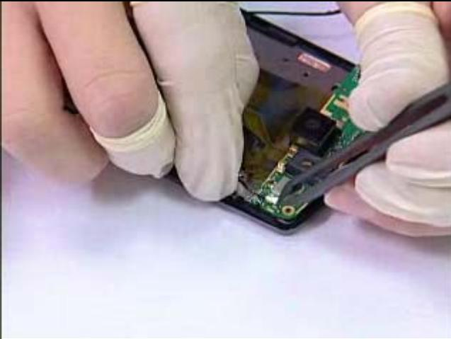
Connect the right coaxial cable GPS with Rigid flex board as shown
