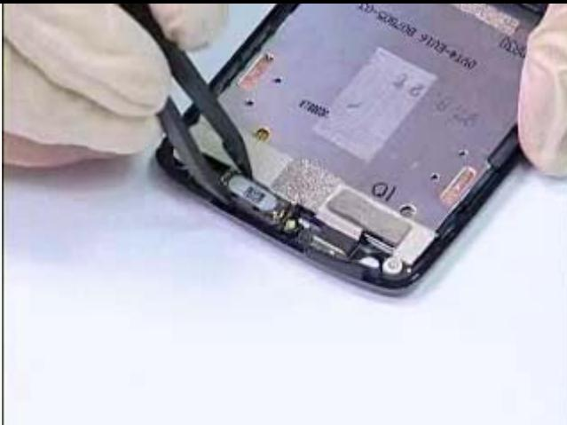
Put the receiver into the slot on the bezel.
