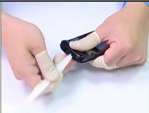
Insert the flat plastic stick between the housing and Antenna cover to release the hooks
