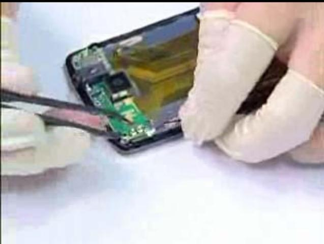
Connect the left coaxial cable BT/WIFI with Rigid flex board as shown
