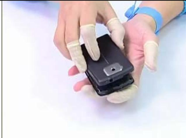
Remove the battery cover as shown
