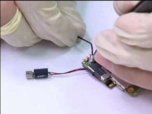
Connect the left coaxial cable BT/WIFI on M/B as shown.
