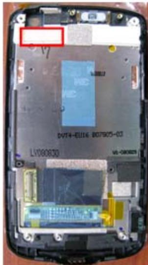
Remove the release paper of the adhesive tape on the bezel as shown
