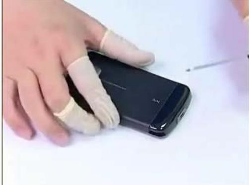
Insert the stylus into the slot
