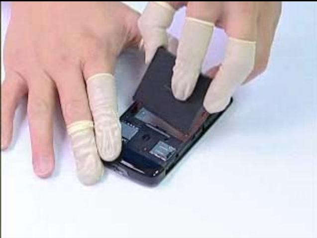
Put the battery into unit as shown
