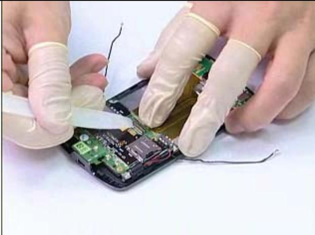
Remove the FPC connector as shown
